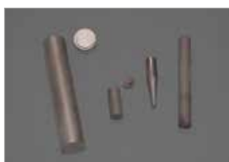
Graphite crucibles for Bridgman growth
