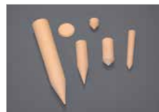
Ceramic crucibles for Bridgman growth
