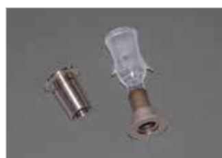
Glass-metal transition pieces for vacuum connection
