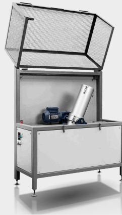
CSR - Coke Strength after Reduction I-Tester/Tumbler
