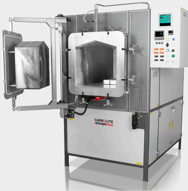
GPCMA /174 fitted with optional compliance to AMS2750G class 1 / type A
