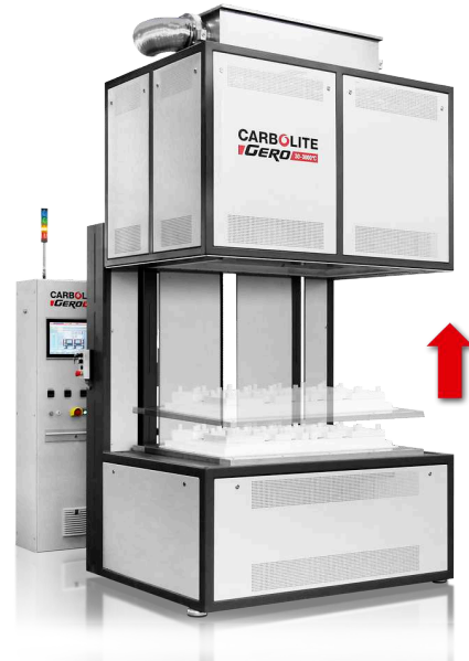
HB-BL 17/430 bottom loader with optional PLC and 19 inch touchscreen control and gas outlet connection to optional catalytic after burner
